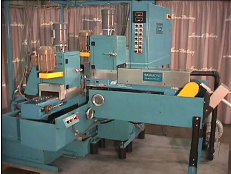
(2) Head Planetary Finishing Machine with Part Flip-over , Coolant Recirculation, Drying, and Demag
